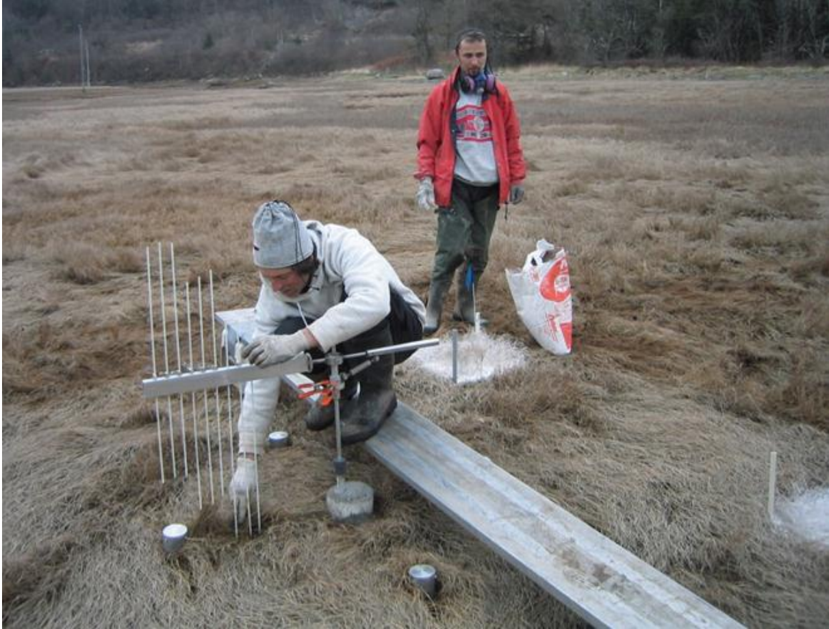
Figure 5.1. Establishing marker horizons at an SET sample station (Dipper Harbour, NB, Canada).
