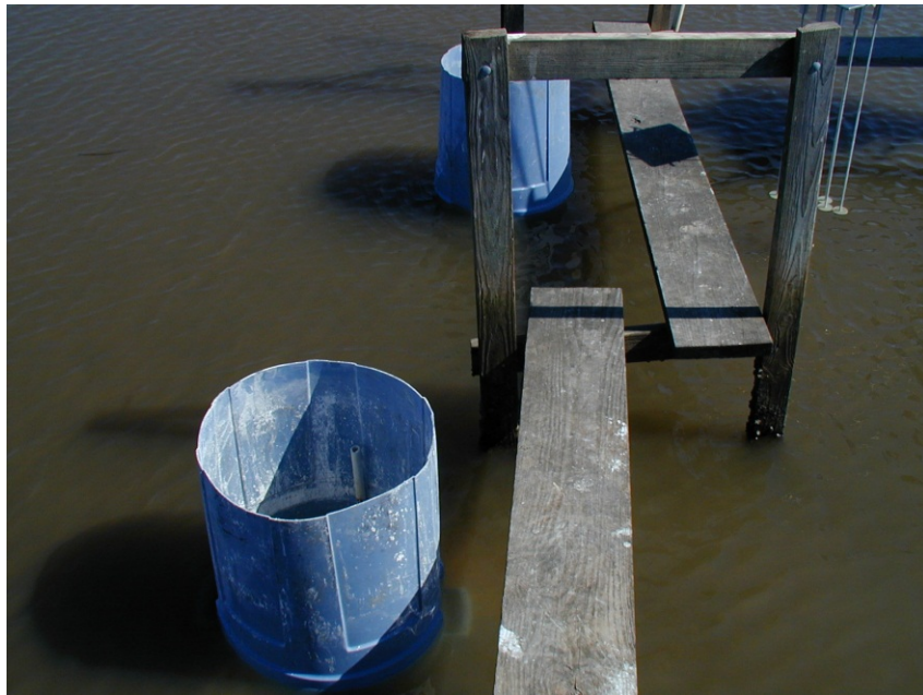
Figure 5.6. Feldspar marker horizon plots established using trash cans in a shallow pond with about 8” (20 cm) of water (Delta NWR, Venice, LA USA).
