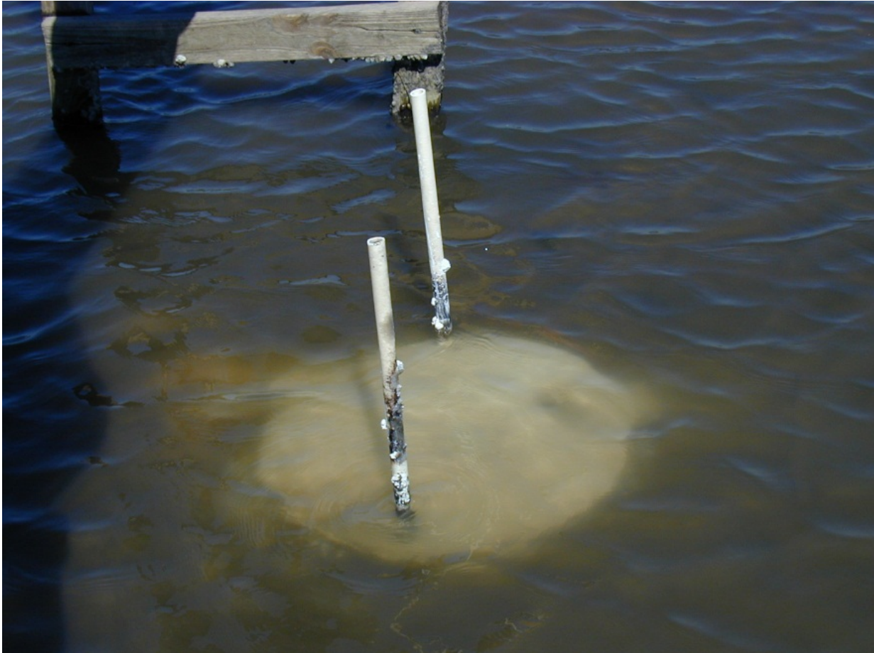
Figure 5.7. Feldspar marker horizon after removing the trash can (Delta NWR, Venice, LA USA).
