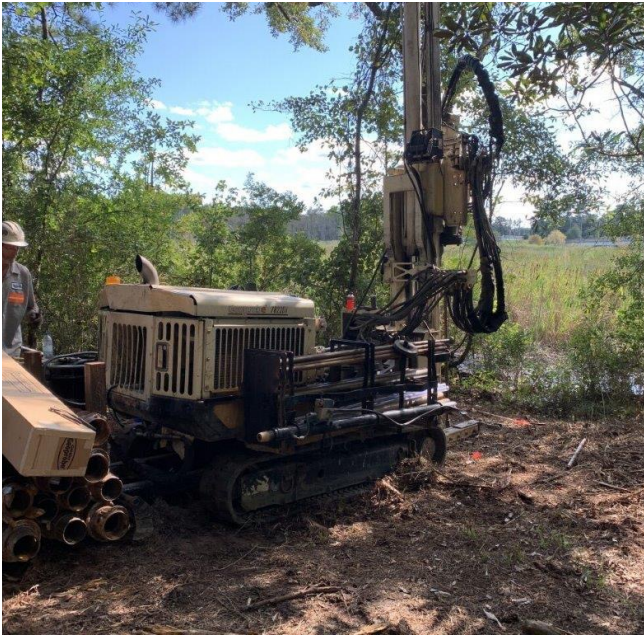
Geoprobe for Soil Boring, Sept 2023
