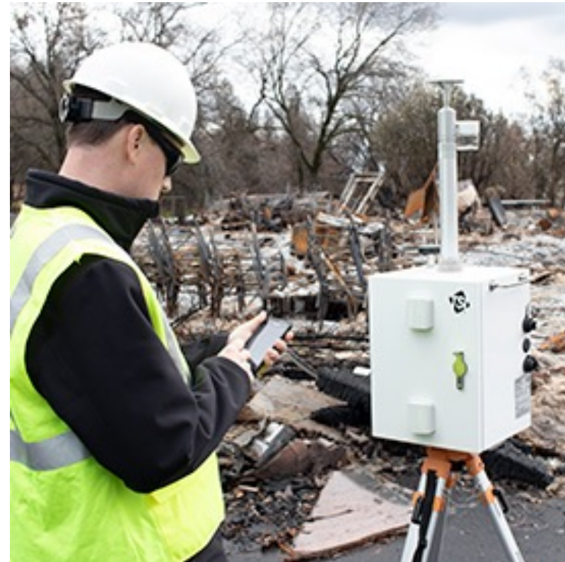
Example Air Monitor - Thermo 1500 TSI DustTrak
